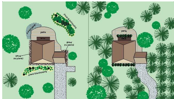
16 Well-designed landscaping (left) can be attractive and will also help keep fire away. Landscaping that is not FireSmart (right) could allow crown fires and surface fires to reach the house. Illustration by Annika Sargent, UW-Extension Environmental Resources Centre.
